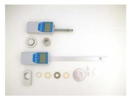
In this picture you see the single parts of the calibration device and a vial with the humidity standard next to an RH5 and an RH1.
